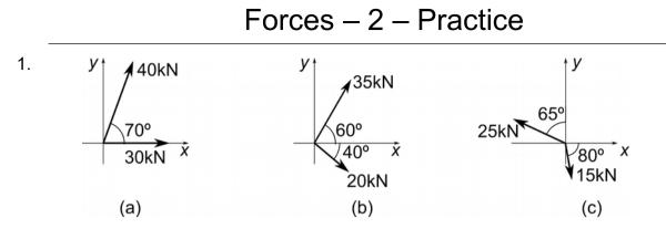
For each of the diagrams a, b, c, calculate the size and direction (relative to the +ve x-axis) of the resultant of the two forces. (58kN, 41°; 37kN, 28°; 20kN, 192°)
