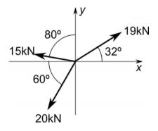
3. Calculate the resultant force acting on the eye bolt. (1.1kN, 88°)
